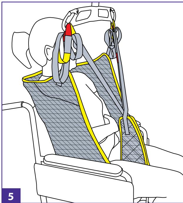
Once the sling has been fitted correctly to your patient attach the appropriate shoulder & leg strap loops to the spreader bar on lift. Color coding on the pick up loops are provided for ease of reference and position. Ensure all straps are attached securely.
