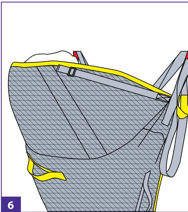
If head support is provided, adjust the head support strap to a suitable position. Ensure the head support cradles the patient's head with the maximum support possible.
